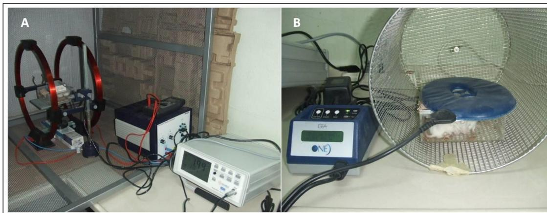
**Fig. 1:** System for generating ELF-EMF: (a) Helmholtz coil exposure set up. (b) Pulsed EMF exposure set up
